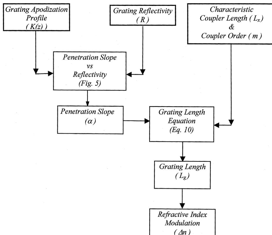
Fig. 6. Grating design algorithm for optimum inscription in a multiple HCC.
