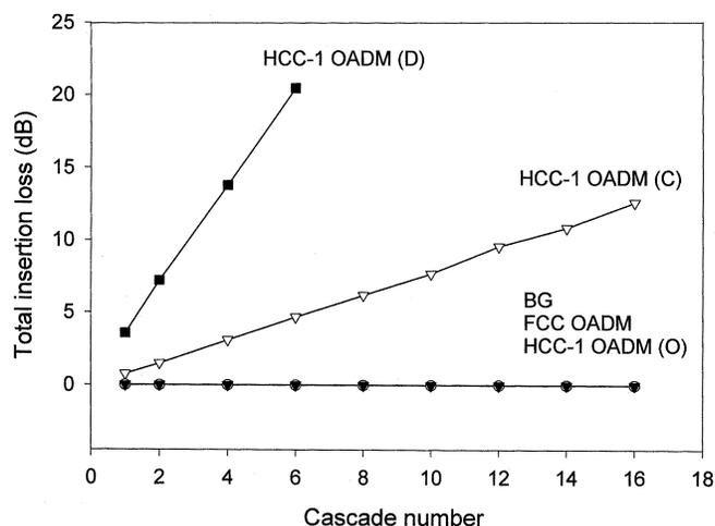
Fig. 13. Comparison of insertion loss for HCC and FCC OADMs in a cascaded filtering operation.
