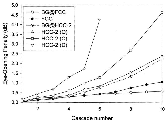
Fig. 12. Comparison of EOP performance between the HCC-2 OADM and the FCC OADM for cascaded filtering. EOP is estimated at 40 Gb/s as a function of the number of the perfectly aligned cascaded filters.
