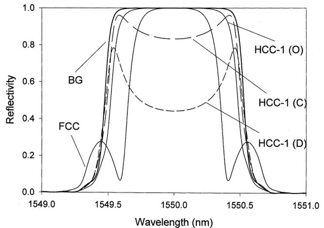
Fig. 10. Reflectivity spectra of the HCC-1 OADM for the optimized (O), compromised (C), and degraded (D) add-drop actions of a half-cycle-based OADM. Also shown is the reflectivity spectrum of the deployed grating (BG).
