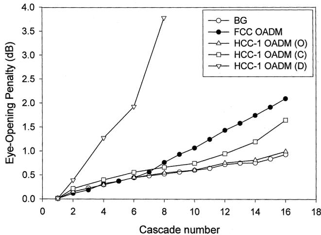
Fig. 14. Comparison of EOP performance between the FCC OADM and the HCC-1 OADM as a function of the number of cascaded filters. EOP is estimated for 40-Gb/s operation, and the cascaded filters are considered perfectly aligned to each other and to the center frequency of the signal spectrum.
