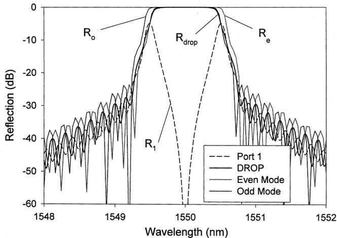
Fig. 2. Spectral response of the HCC-based OADM. The drop action is formed by the partial overlap of the even and odd modes reflection spectra.
