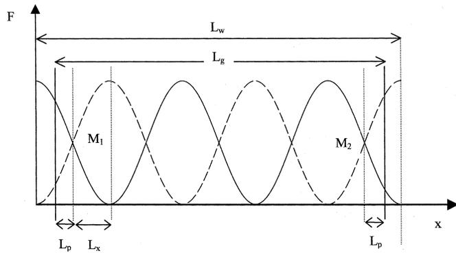
Fig. 4. Schematic of the optimum arrangement of a Bragg grating in a multiple HCC (here  $m = 5$ ).
