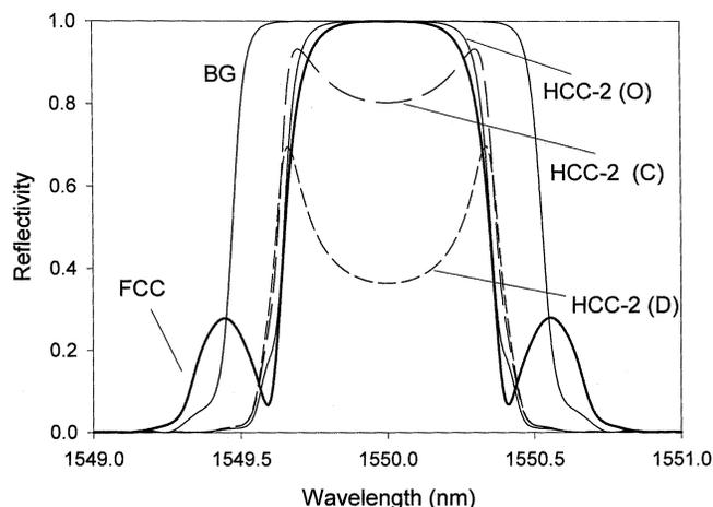
Fig. 11. Reflectivity spectra of the HCC-2 OADM for the optimized (O), compromised (C), and degraded (D) add-drop actions. Also shown, for comparison, is the reflectivity spectrum of the FCC OADM. The optimized response (O) of the HCC-2 OADM and the FCC OADM exhibits the same 3-dB bandwidth of 0.7 nm.
