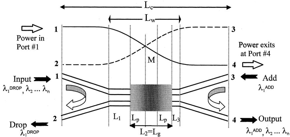
Fig. 1. Schematic of the half-cycle coupler (HCC) OADM with the power evolution along the full coupler. The OADM is configured in an asymmetric configuration for optimized drop action.
