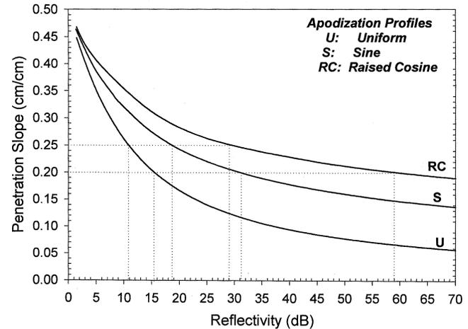
Fig. 5. Engineering curves for penetration slope versus reflectivity for various apodization profiles.
