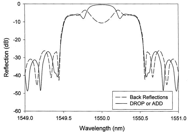
Fig. 9. Spectral response of a nonoptimally designed FCC OADM. The deployed grating is of optimum length 4.5 mm as in Fig. 6, but its reflectivity is only 25 dB.
