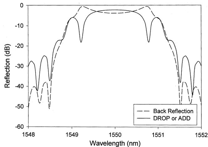
Fig. 8. Spectral response of a nonoptimally designed FCC OADM. The deployed grating exhibits the required reflectivity 45 dB, but the length is 2.5 mm.
