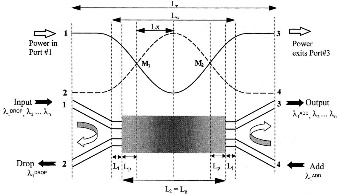
Fig. 3. Schematic of the FCC OADM with the power evolution along the full coupler. The configuration of the device is symmetric for optimized add-drop actions.
