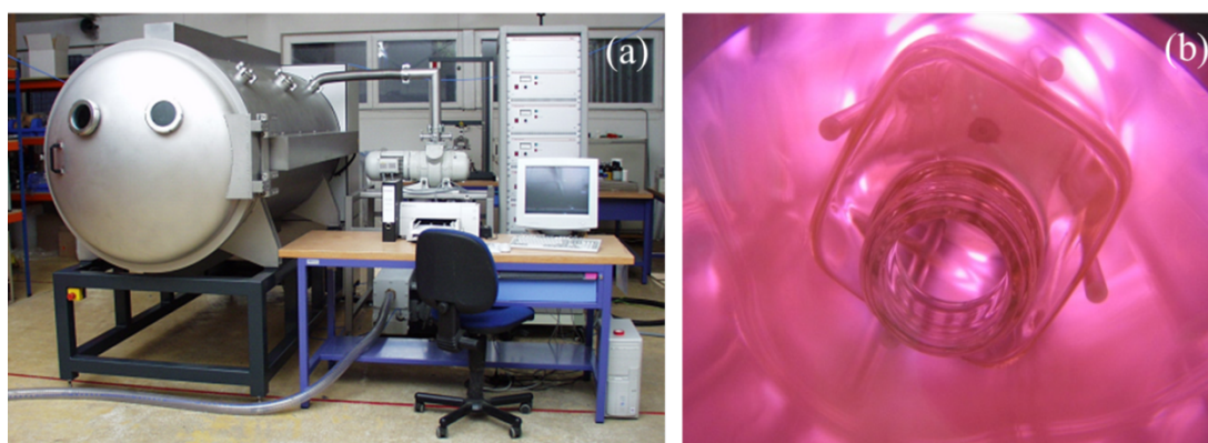
Figure 5.1 (a) Photograph of Microwave plasma device used during the study, (b) glass drum with the excited microwave plasma.
