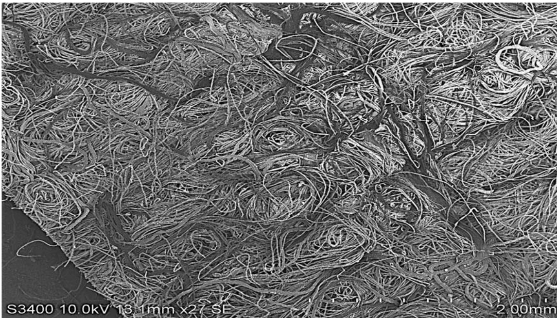
Figure 4.55b SEM of calendared hydroentangled nonwoven fabric S11 showing structure of the fabric.
