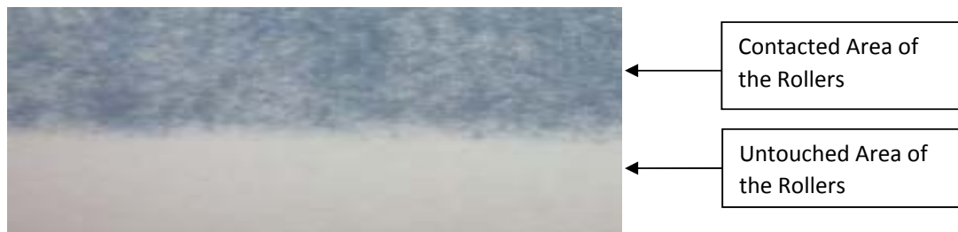
Figure 3.8 Carbon paper showing roller contact
