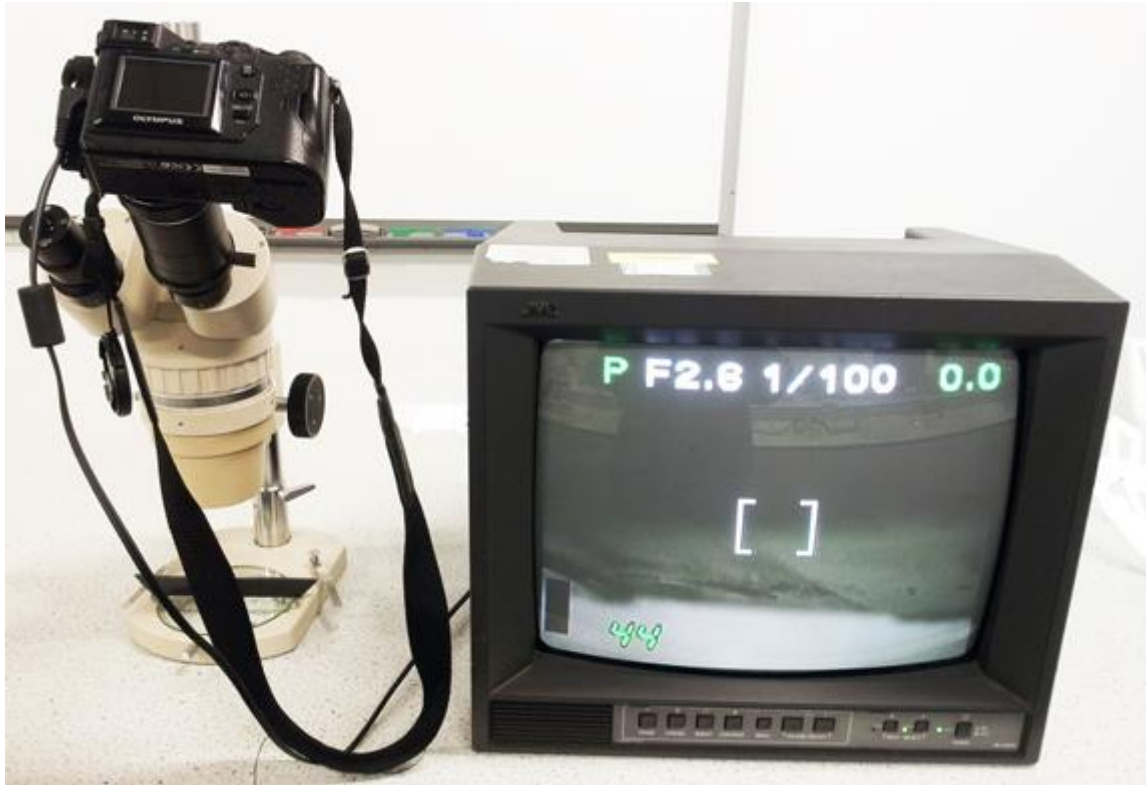
Figure 3-14 Damage inspection set-up apparatus
