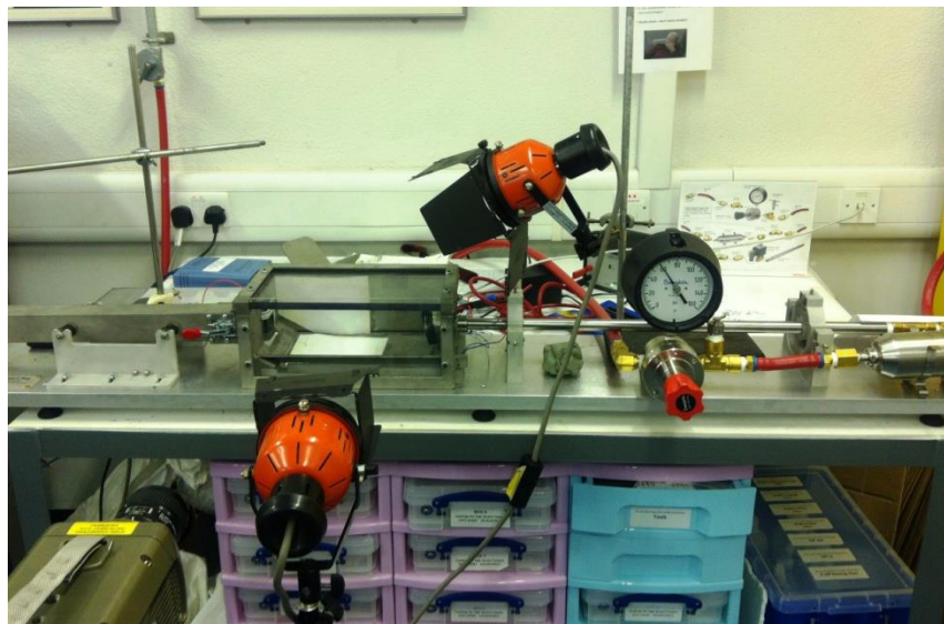
Figure 3-12 High velocity impact testing rig
