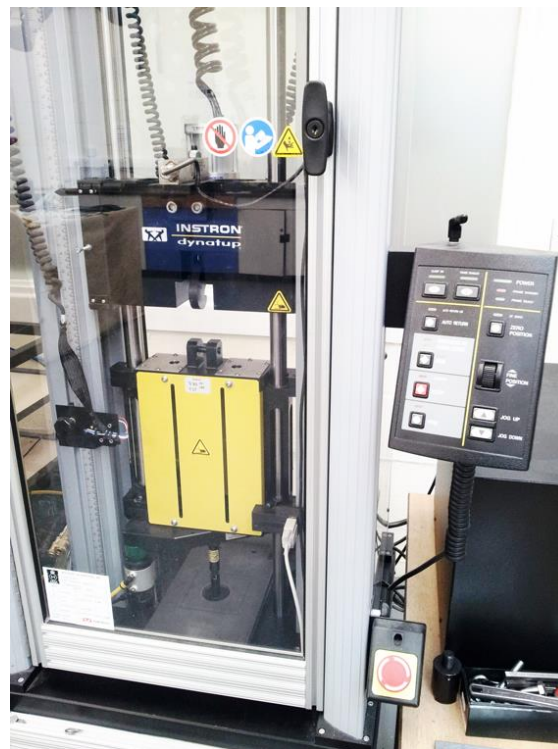
Figure 3-11 Instron Dynataup® Model 9250HV Drop Tower Impact Tester
