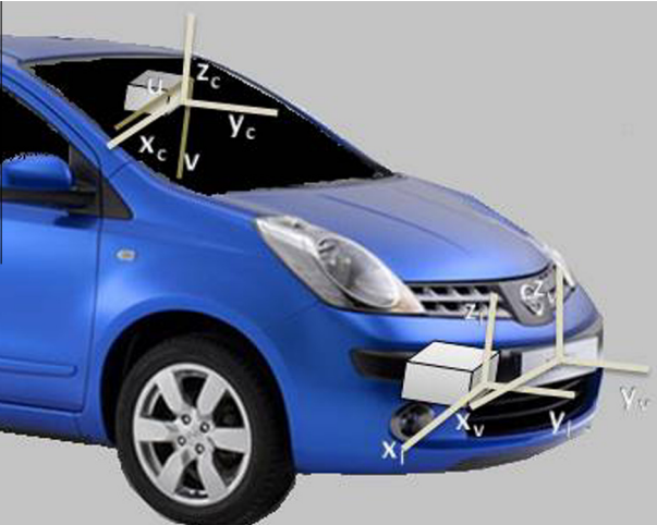
Fig. 9. Different coordinate system (x_c, y_c, z_c) are camera coordinate system, (x_l, y_l, z_l) is the laser coordinate system, and (x_v, y_v, z_v) is the coordinate system. Coordinates (u, v) are the image coordinates.
