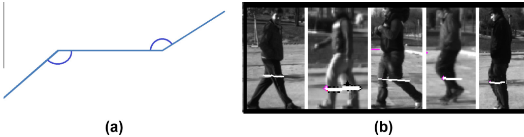
Fig. 8. (a) Pattern for pedestrian detection. (b) Different examples of different patterns given by pedestrians with different leg positions.
