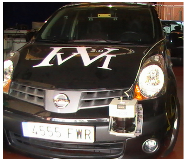
Fig. 4. Platform IVVI 2.0 with the laser scanner mounted in the front bumper and the computer camera system in the windshield.
