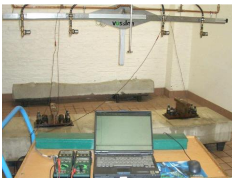
Fig.3. Determining the electrical resistance in wet conditions, in laboratory
