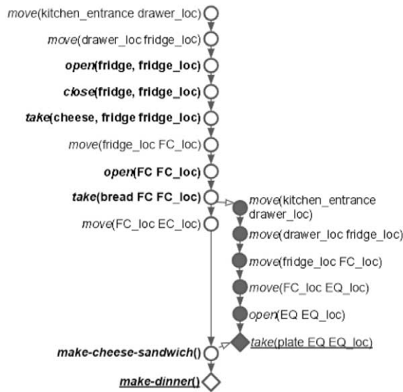
Fig. 12. The order the human performs actions when their goal is to make dinner (left) and the actions executed by the robot (right) when its initial location is kitchen_entrance . With the following parameters: \theta = 0.85 , \beta = 0.45 , w = 0.5 .
