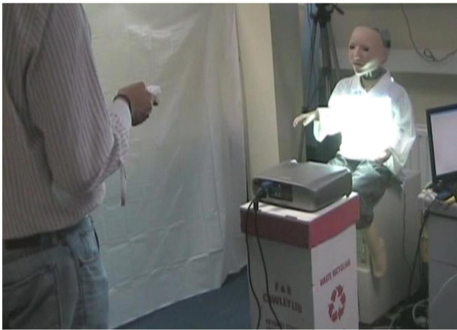
Fig. 2. Experimental layout: in the human-humanoid experiment, a participant was instructed to stand in front of KASPAR2 and hold a Wii Remote to perform a gesture pattern. The trajectories produced were projected onto the body of KASPAR2 using a projector.
