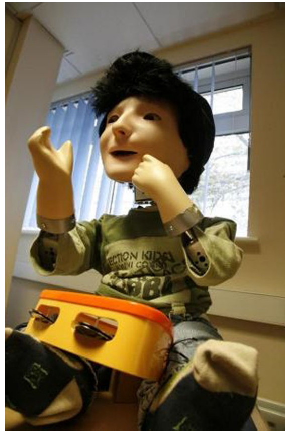
Fig. 1 KASPAR is a child-sized humanoid robot and was developed to study human-robot interaction by the Adaptive Systems Research Group at the University of Hertfordshire
