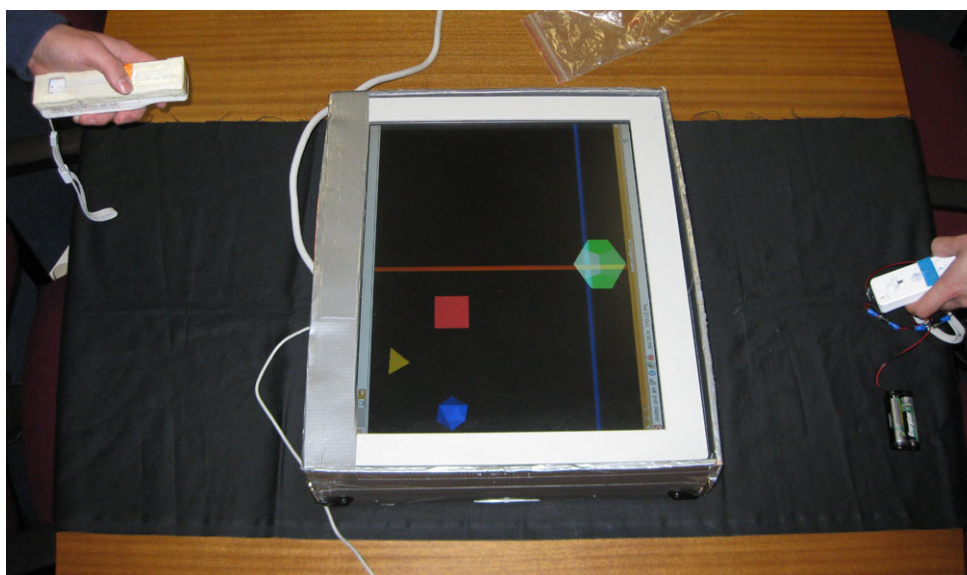
Fig. 2 The dyadic collaborative game. The player on the left (stand-in for the child with autism) controls the location of the orange selection line , while the player on the right (stand-in for the human adult or the humanoid robot) controls the location of the blue selection line (Color figure online)
