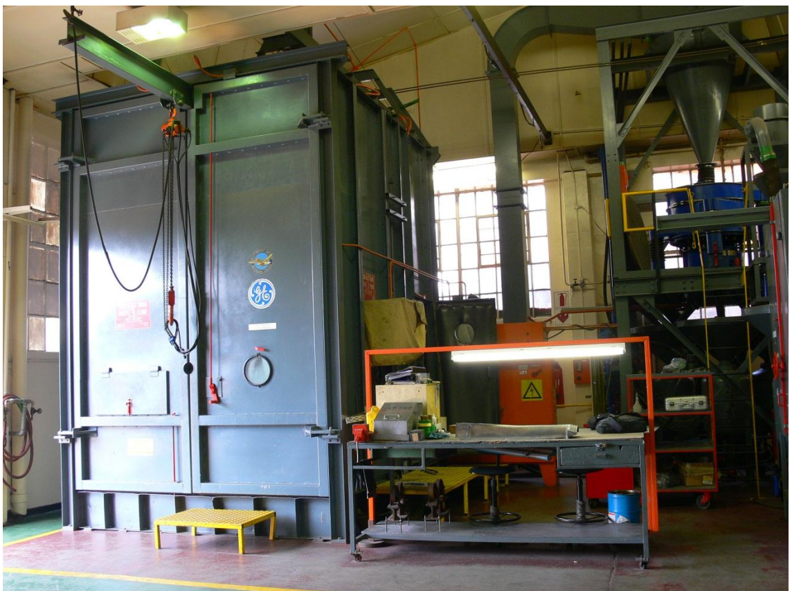
Figure 48: Shot Peening chamber at South African Airways Technical Services
