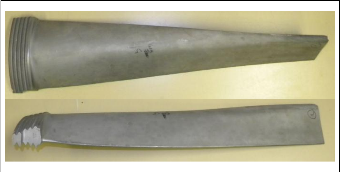
Figure 5: Complete last stage LP turbine blade
