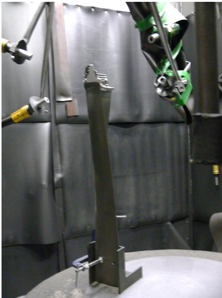
Figure 49: Turbine blade mounted on turn table inside shot peening chamber
