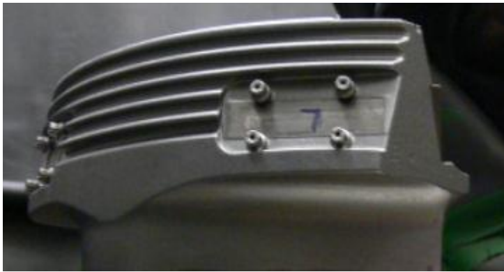
Figure 21: Almen strip location on old turbine blade with a fir tree root
