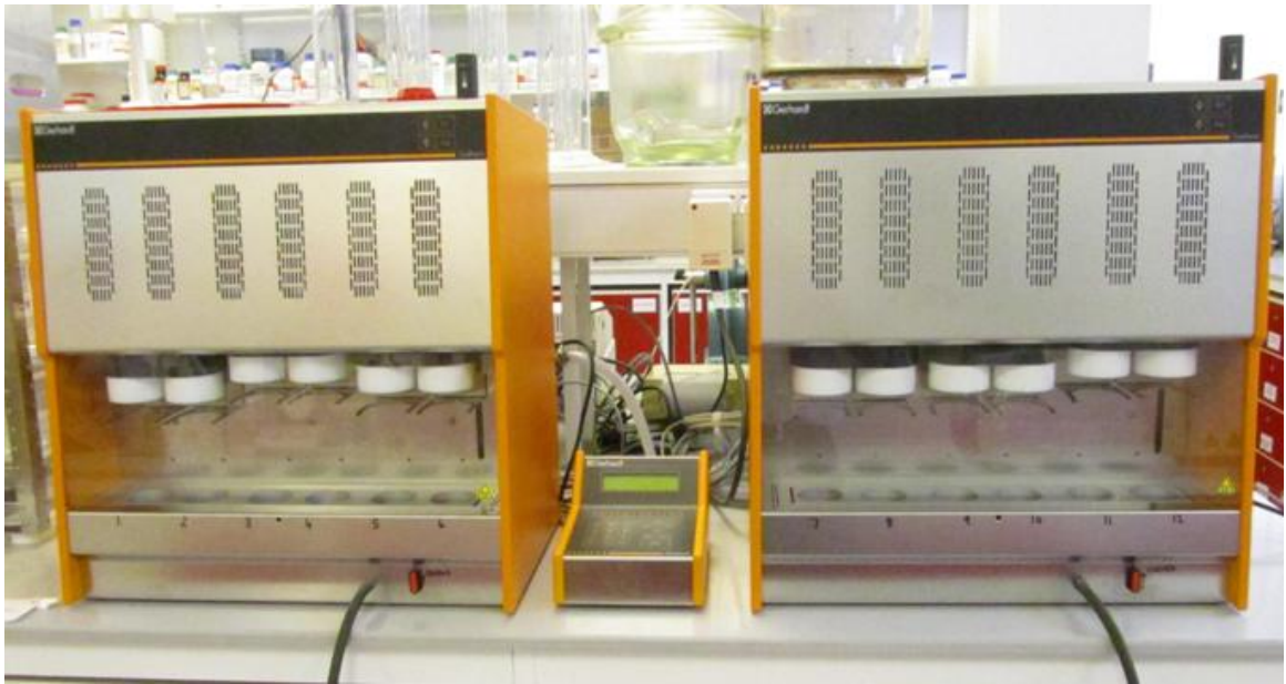
Plate 2.4 Soxhlet system operated in the nutrition laboratory of the University of Plymouth.
