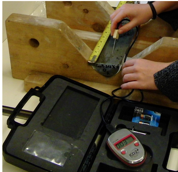
Fig. 6.5.3: Needle probe applied to a split core. A Decagon KD2 physical property analyzer is used for measurements.
