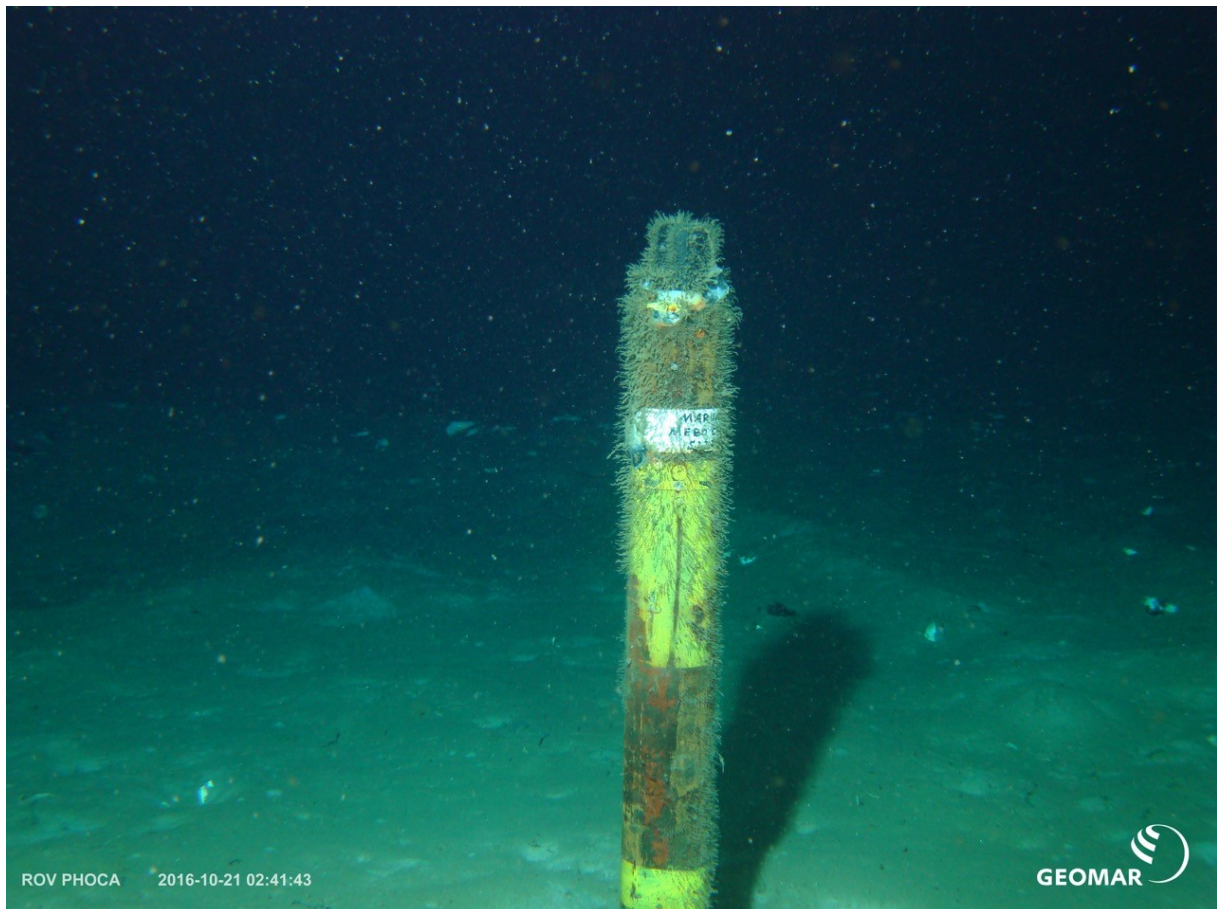
Fig. 7.2.2: Former MeBo hole with end cap once CORK-B was recovered in 2012 (Kopf et al., 2013).
