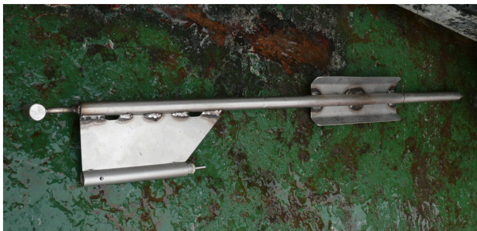
Fig. 6.3.3: MTL stick to be deployed by ROV; those systems complement the MeBoPlugs at two sites to get high-resolution seafloor temperature variations as reference for the MeBoPlug data. ROV handle is seen left, MTL is hosted in a metal tube; lower portion is stuck into the sediment (with metal shield for stabilisation in case of bottom currents).
