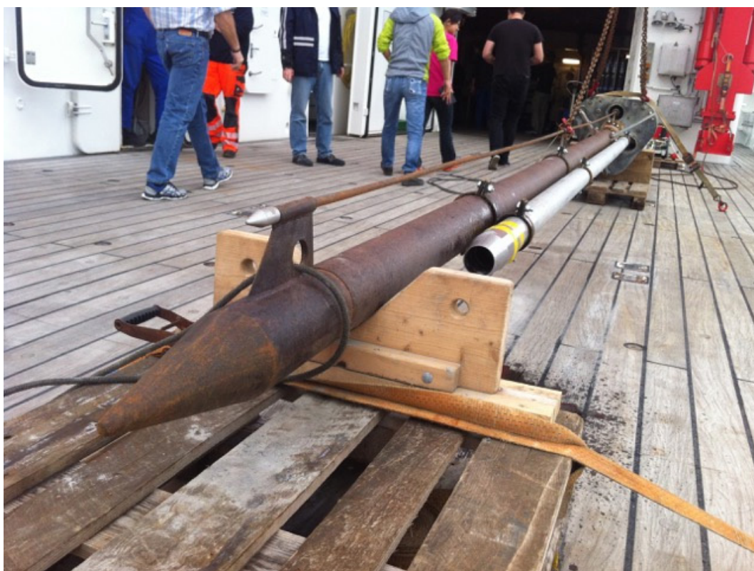
Fig. 6.4.3 The new „Heat flow corer“, an improvised sampling device developed on board, on deck before being deployed in the Kumano Basin.
