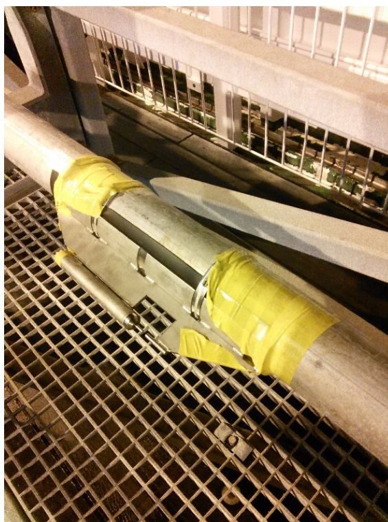
Fig. 6.7.1: Photo of MTL sensors mounted onto the core barrel
