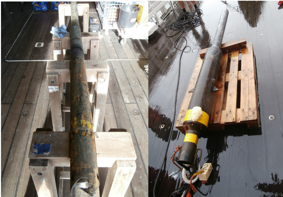
Fig. 7.3.3. MeBo CORK A borehole rod and SmartPlug deployment configuration once safe on deck.
