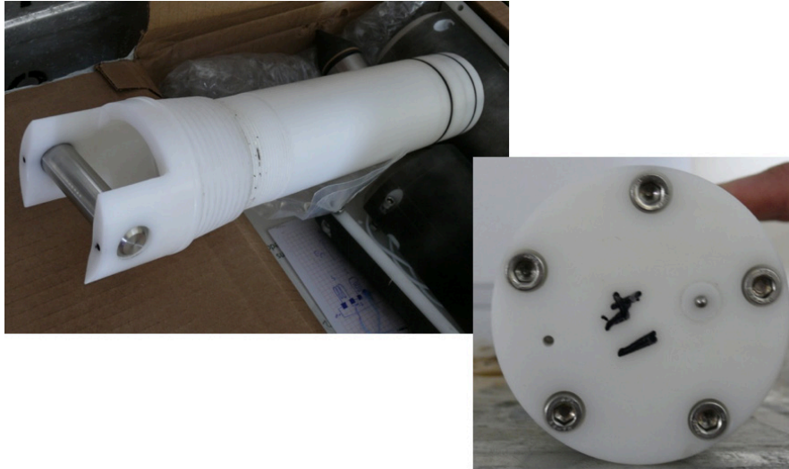
Fig. 6.3.2: MeBoPlug prior to being screwed into a MeBo drill pipe (left); right image shows bottom view into the borehole with ports for P [hole at left] and T [little pin at right] monitoring. See text.
