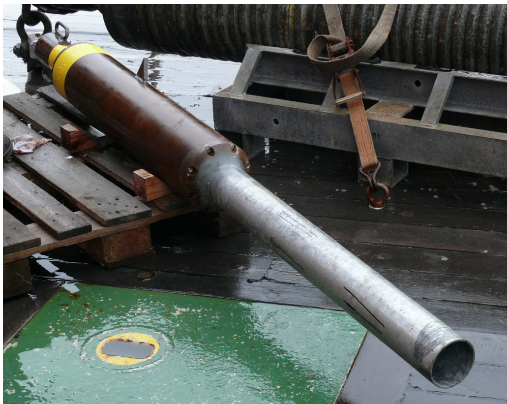
Fig. 6.3.4: SmartPlug converted into a piezometer before being mounted to the TV-grab for deployment.
