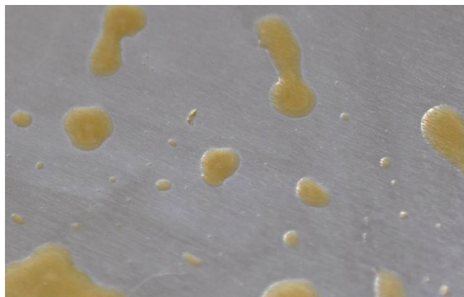
Figure 50: Cured mixture of resin and dibutyl sebacate on pretreated aluminum wafer with Bayer release agent
