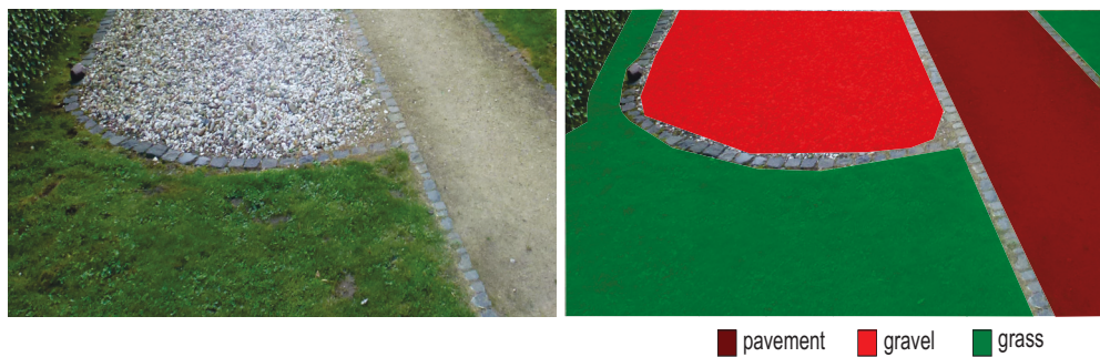
Figure 8.39: Camera image containing multiple terrain types (left) and its color coded hand labeled ground-truth image (right).
