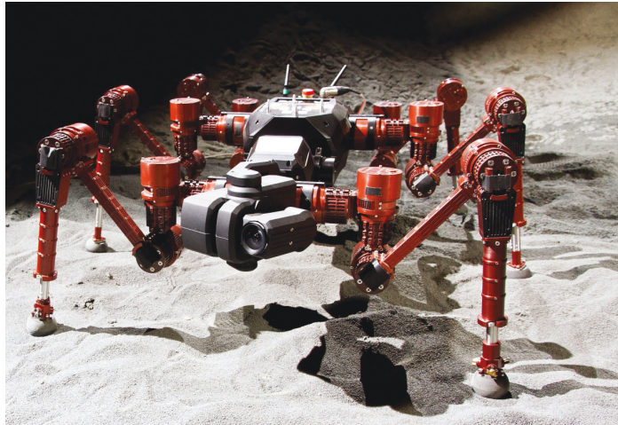
Figure 3.6: CREX the legged robot used in the context of this research.
