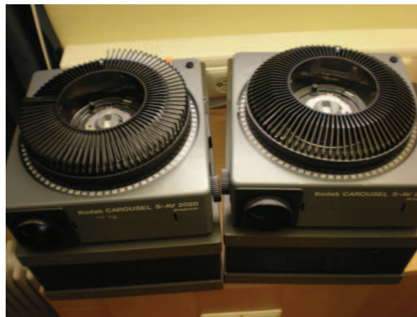
Figure 2.3: The two Kodak carousel-projectors of the tachistoscope
