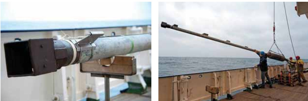
Fig. 49: The core catcher with lids and the lowermost T-Logger (left). Deployment of the gravity corer equipped with a 6 m long steel barrel and T-loggers (right).
