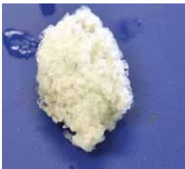
Fig. 82: Very porous, white gas hydrate with sediment of Helgoland MV (GC-41; GeoB15525-1; photo: SL_GeoB_15525_1_VD15910.JPG). Length of aggregate about 3 cm.
