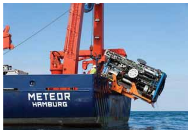
Fig. 2: Research vessel METEOR on mission in the Black Sea (left). Launching of the mobile drilling system from R/V METEOR during M84/2 (right).
