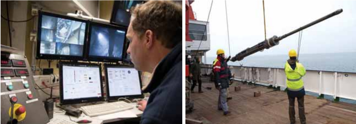
Fig. 3: View inside the control container during drilling a MeBo drill site (left). The Dynamic Autoclave Piston Corer during the deployment onboard R/V METEOR (right).
