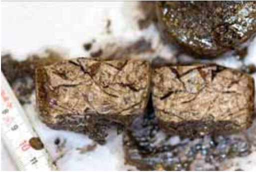
Fig. 70: Internal structure of gas hydrate from Pechori Mound drilled by MeBo (MeBo-67; GeoB 15227-3 8R-2A 96-106cm; photo: _VD14055).
