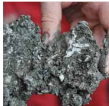
Fig. 75: Dispersed hydrates in core GC-17 taken at the Batumi seep area (GeoB 15252; photo _DSC2206).
