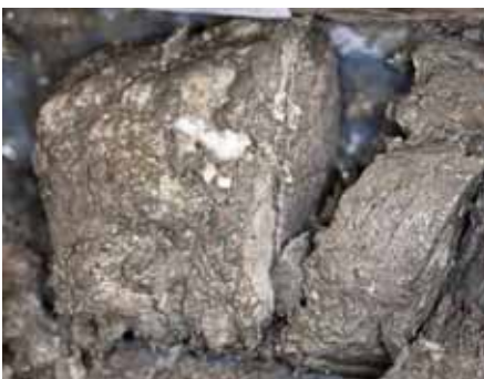
Fig. 76: Massive 10 cm-thick gas hydrate at the base of GC-11 (~130-140 cm) taken at Poti Seep (GeoB 15244-2; photo: _VD14412).
