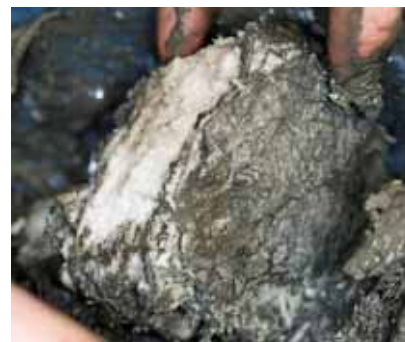
Fig. 77: Massive gas hydrates recovered with GC-11 from Poti seep (GeoB 15244-2; photo: _VD14416).
