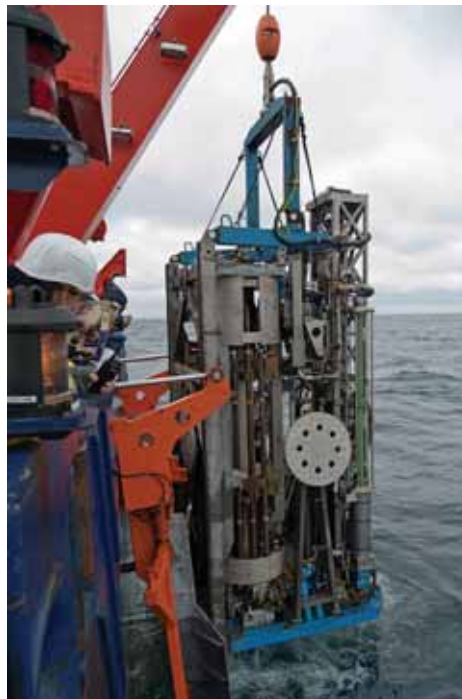
Fig. 42: The sea floor drill rig MeBo during the first deployment of expedition M84/2 (picture).
