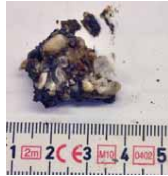
Fig. 71: Porous gas hydrate from Pechori Mound recovered with GC-21 (Geo B15256; photo _DSC2268).
