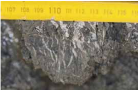
Fig. 74: Finely laminated hydrates in core GC-16 from the Batumi seep area (GeoB 15251-1; photo: _VD14763).
