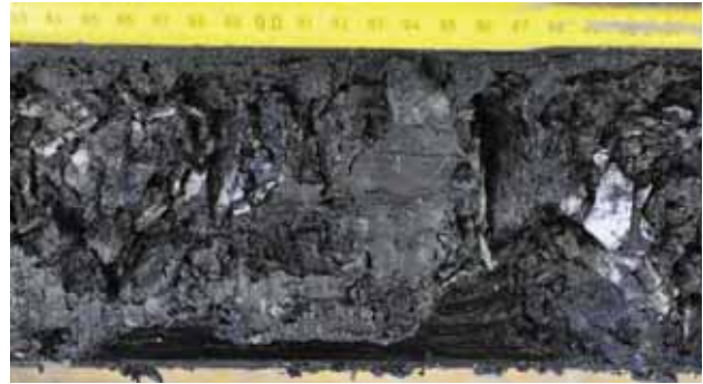
Fig. 81: White gas hydrate plates in black sediments at Kerch flare (GC-36; GeoB15516-1; photo: 74-104 GH 7).
