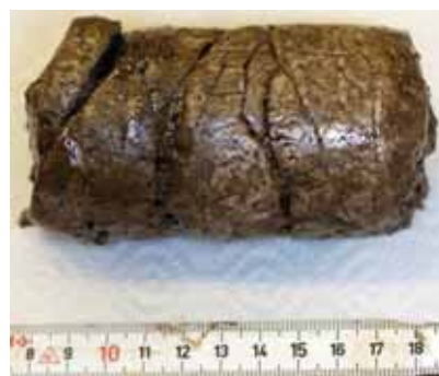
Fig. 69: Massive gas hydrate from Pechori Mound drilled by MeBo (MeBo-67; GeoB 15227-3 8R-2A 96-106cm; photo: _VD14033). Core diameter 55 mm.
