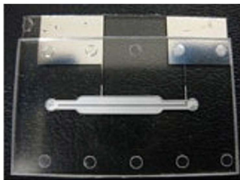
Fig. 4 Final prototype developed by the Ahn and Bishop groups 12 for the analysis of Pb(II) and Cd(II). Reprinted from ref. 12, with permission.
