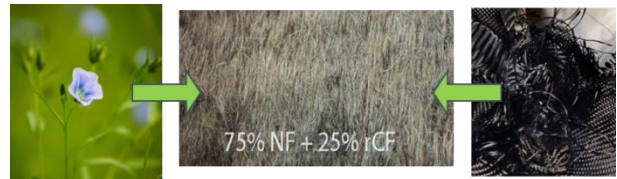
Figure 6: Combination of flax fibres and recycled carbon fibres in a hybrid non-woven
