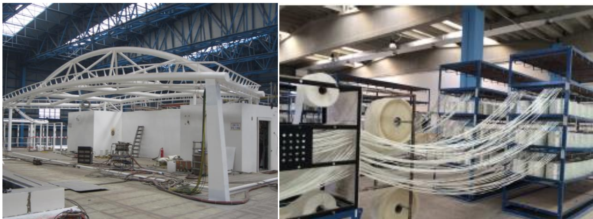
Fig. 4 (a) typical superstructures and walls on a cruise vessel; (b) preparation of fibres for pultruded profiles for RoRo decks
