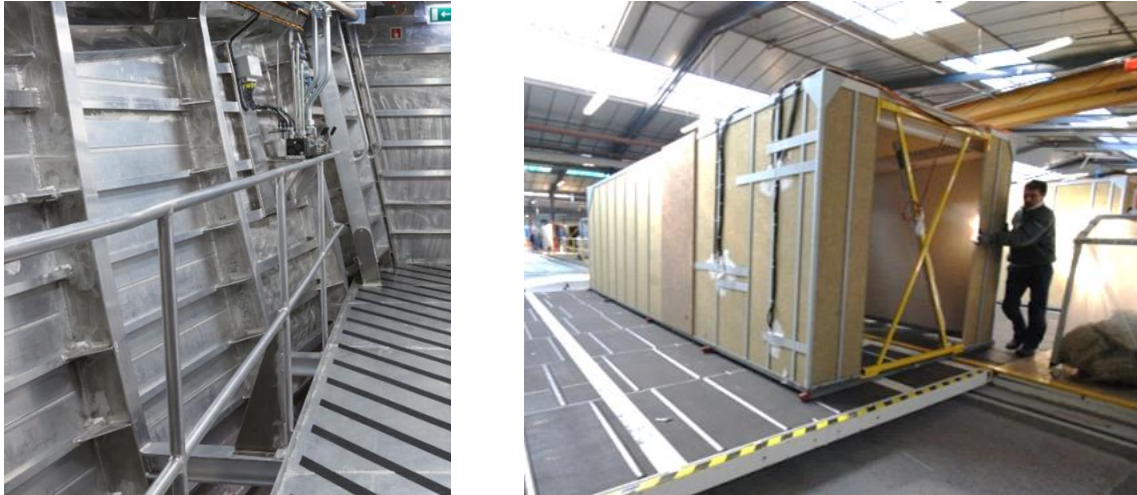
Fig. 5 (a) Extruded Aluminium profiles in a workboat, joined by friction stir welding; (b) Conventional passenger cabins without floor
