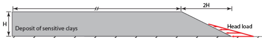
FIGURE 1 Schematic diagram for a deposit of sensitive clays [Colour figure can be viewed at wileyonlinelibrary.com ]
