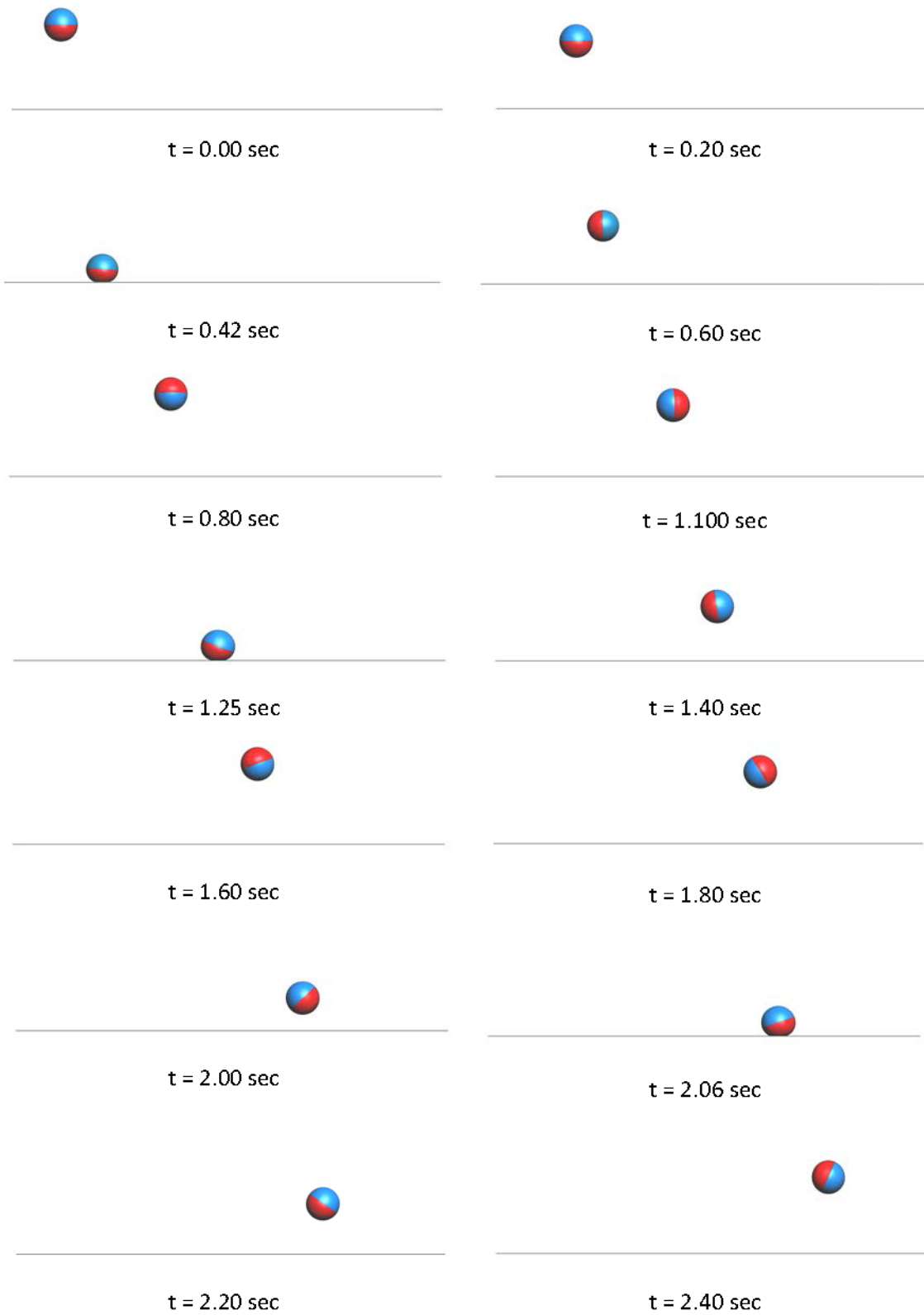
Figure 13. Elastic ball bouncing on a rigid surface. Deformation configuration at different time steps.
