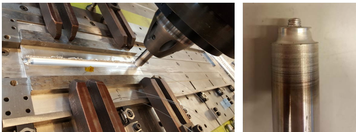
Figure 3. Experimental setting and pin detail
