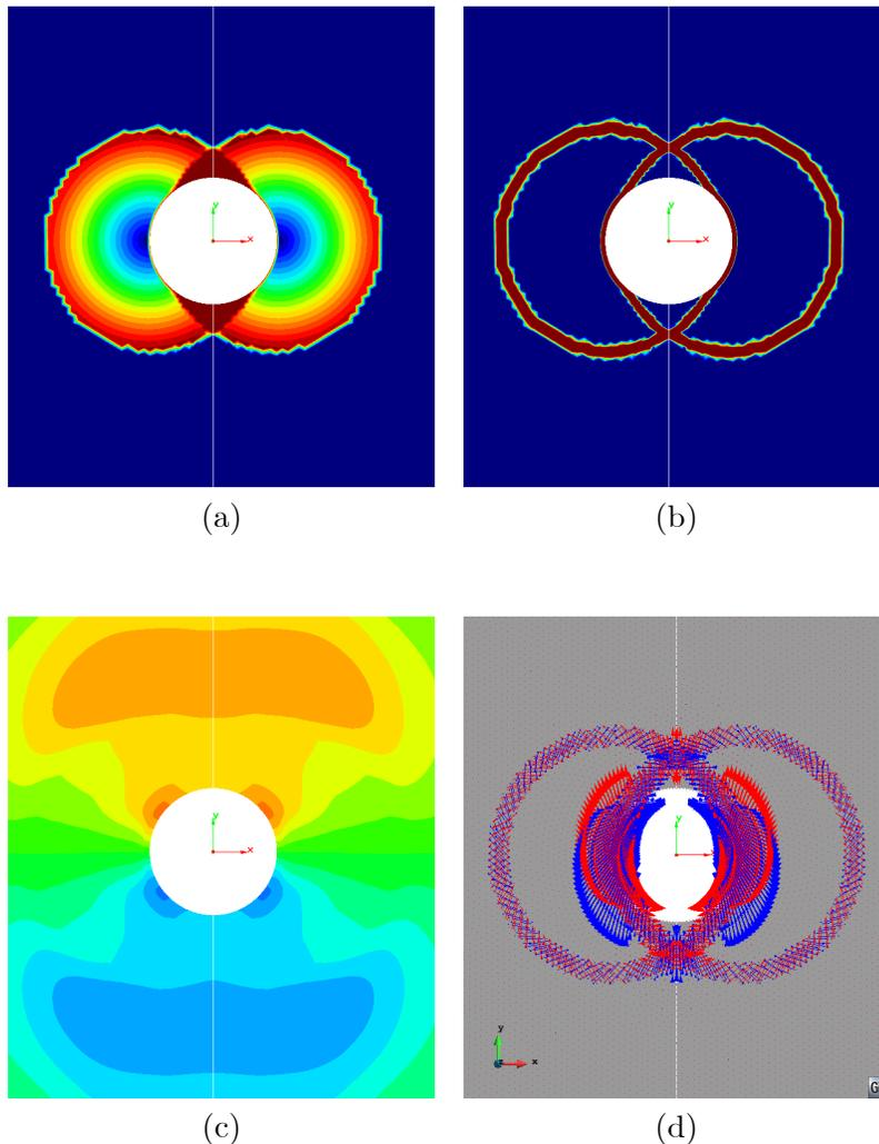
Figure 9: Results for circular rigid inclusion using the mixed  $\varepsilon/\mathbf{u}$  formulation. Incompressible plasticity,  $\phi = 0^\circ$ . Contours for: (a) displacement, (b) equivalent plastic strain, (c) pressure and (d) principal strain vectors
