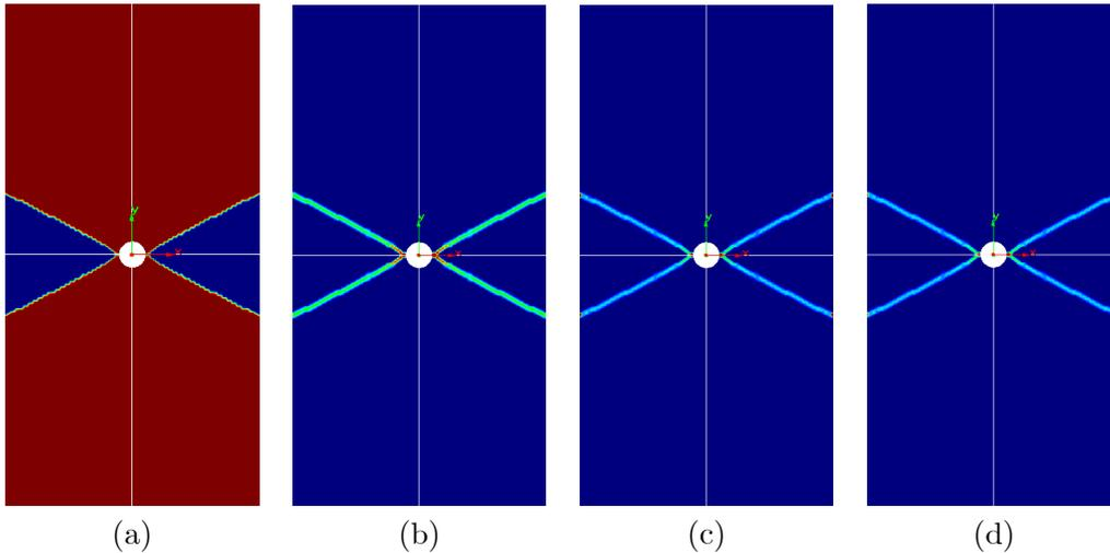
Figure 6: Results for singly perforated strip with the mixed  $\boldsymbol{\varepsilon}/\mathbf{u}$  formulation; compressible case  $\phi = 45^\circ$ . Contours for: (a) vertical displacement, (b) equivalent plastic strain, (c) volumetric plastic strain and (d) deviatoric plastic strain
