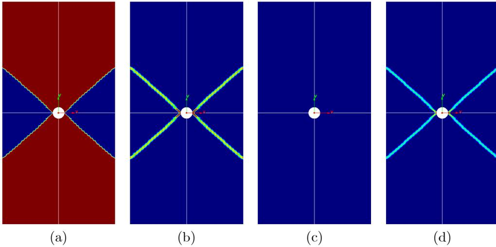
Figure 4: Results for singly perforated strip with the mixed  $\boldsymbol{\varepsilon}/\mathbf{u}$  formulation; incompressible case  $\phi = 0^\circ$ . Contours for: (a) vertical displacement, (b) equivalent plastic strain, (c) volumetric plastic strain and (d) deviatoric plastic strain
