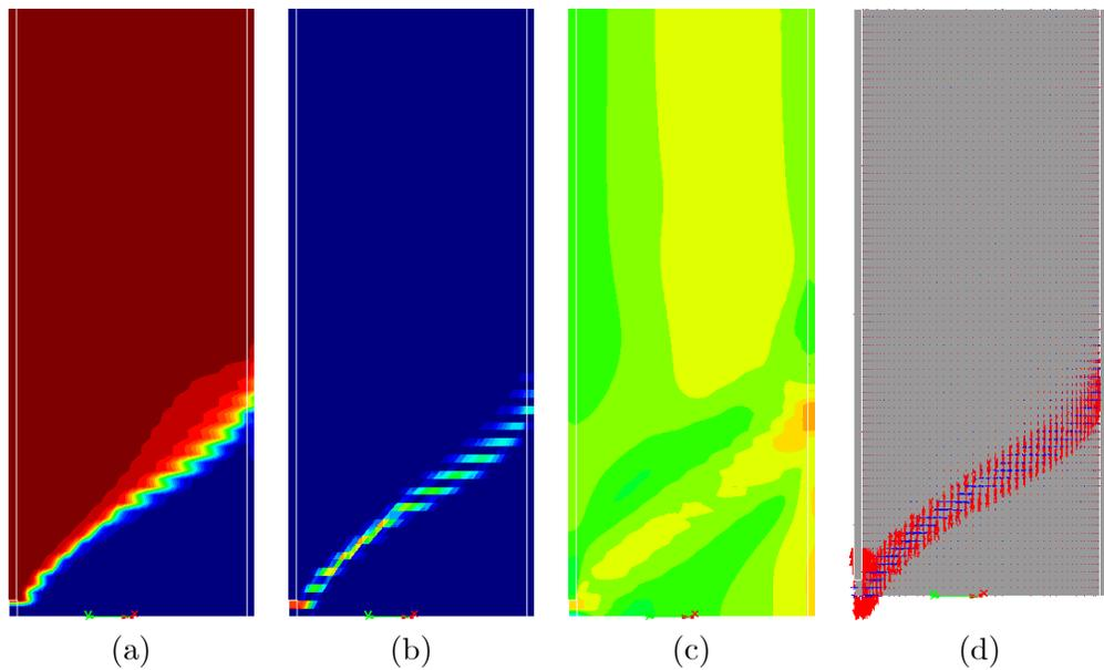
Figure 13: Results for simply perforated thin-walled cylinder with the mixed  $\mathbf{u}/p$  formulation. Contours for: (a) vertical displacement, (b) equivalent plastic strain, (c) pressure and (d) principal strain vectors
