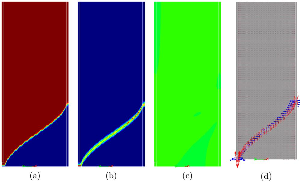
Figure 12: Results for simply perforated thin-walled cylinder with the mixed  $\varepsilon/\mathbf{u}$  formulation. Contours for: (a) vertical displacement, (b) equivalent plastic strain, (c) pressure and (d) principal strain vectors
