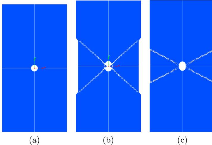
Figure 2: Geometries for the singly perforated strip: (a) undeformed, (b) deformed (x 5)  $\phi = 0^\circ$ , (c) deformed (x 5)  $\phi = 45^\circ$
