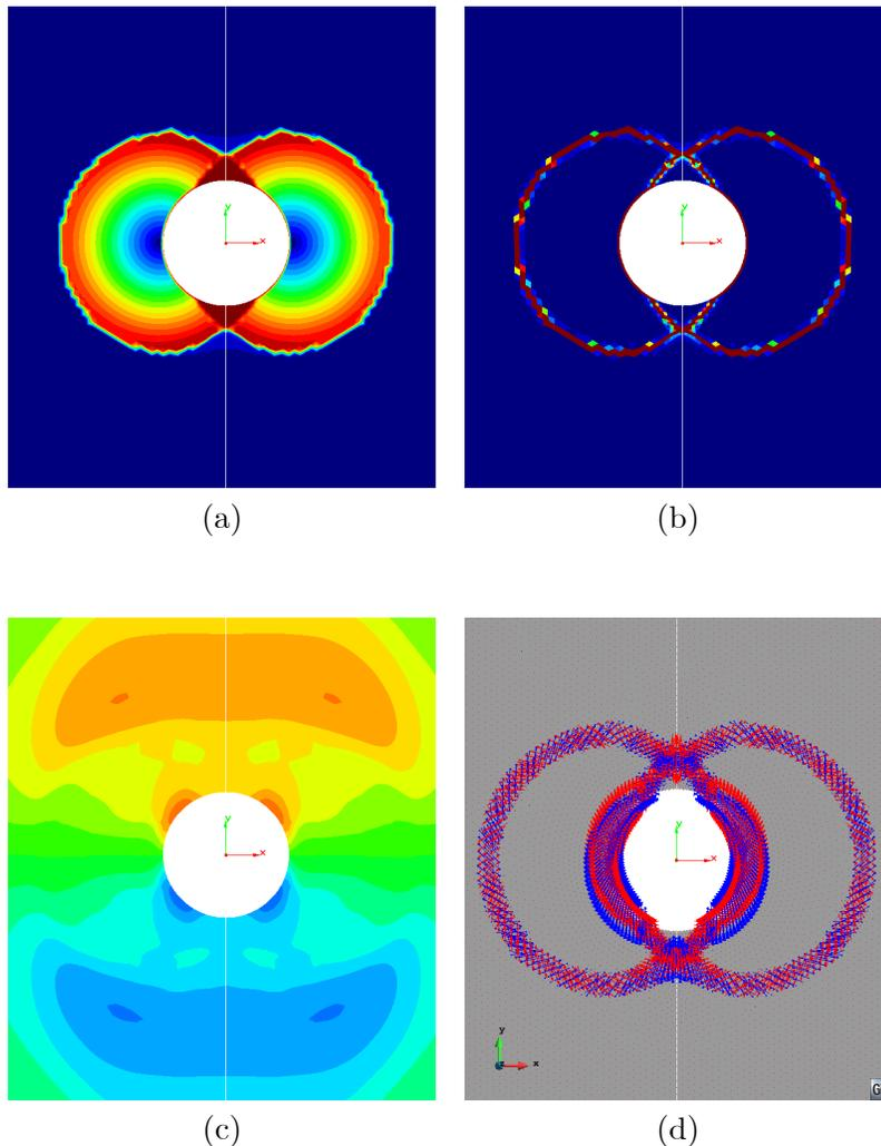
Figure 8: Results for circular rigid inclusion using the mixed  $\mathbf{u}/p$  formulation. Incompressible plasticity,  $\phi = 0^\circ$ . Contours for: (a) displacement, (b) equivalent plastic strain, (c) pressure and (d) principal strain vectors
