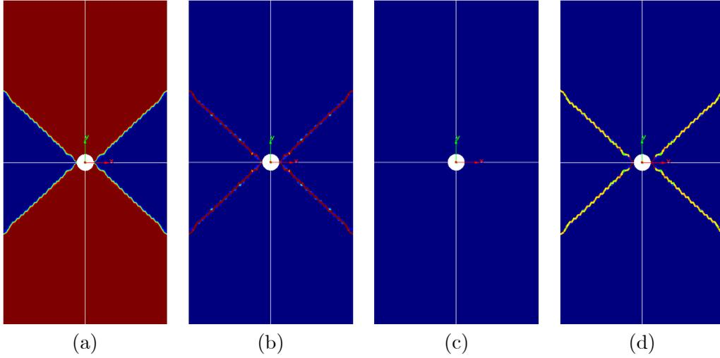
Figure 3: Results for singly perforated strip using the mixed  $\mathbf{u}/p$  formulation; incompressible case  $\phi = 0^\circ$ . Contours for: (a) vertical displacement, (b) equivalent plastic strain, (c) volumetric plastic strain and (d) deviatoric plastic strain
