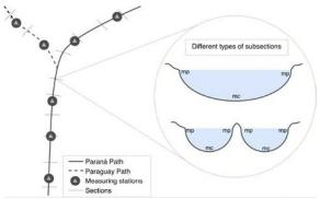
Fig. 1 Discretization of the simulated domain river system.
