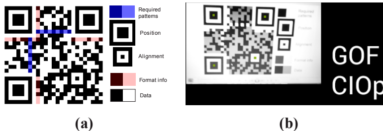
Fig. 3. (a) QR code of the text “GOF CIOp” and (b) the outcome when reading the QR code with a smartphone.
