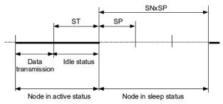
Figure 4: Duty cycle configuration of a XBee node
