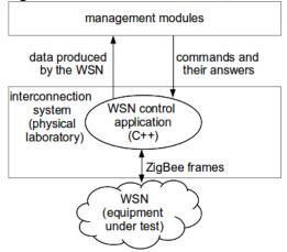
Figure 1: Interconnection system of the remote laboratory prototype based in a traditional implementation
