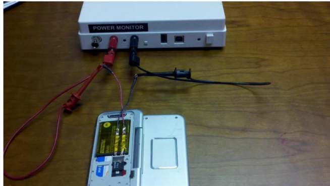
Fig. 4 Power Monitor Setup
