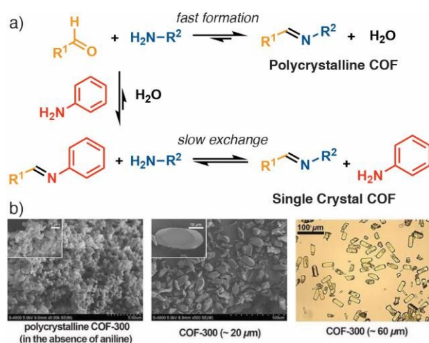
Figure 20. a) Schematic of aniline-modulated self-assembly of imine COFs to modify kinetics. b) Selected SEM and optical images of COF-300 samples illustrating the particle size control offered by modulation. Reprinted in part (adapted) with permission from reference 110. Copyright (2018) The American Association for the Advancement of Science.
