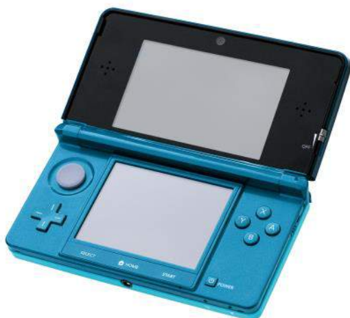
Figure 2. The Nintendo 3DS uses parallax barrier autostereoscopy to display a 3D image.
