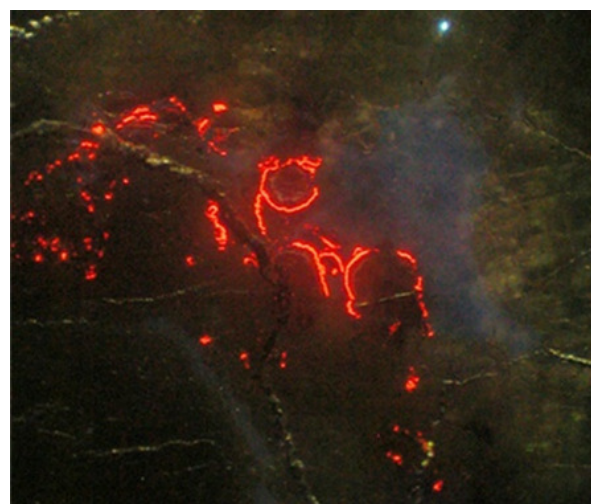
Figure 2. Cathodoluminescence image obtained of the D5 ROI in Fig. 1 (note the curved crack for further identification) using an accelerating voltage of 20-24 keV. As Fe is a typical quencher, the right red areas correspond to Fe-poor and Mn-rich carbonate layers that nicely delineate the carbonate globule walls.
