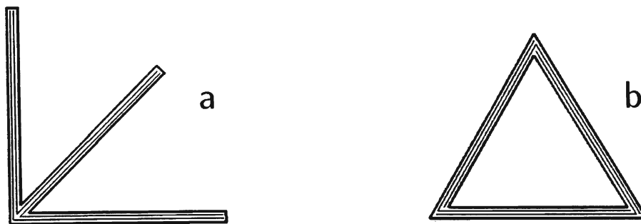
Figure 8.1: Schematics of two configurations with three interferometers at one site: a. rectangular, with bisector; b. equilateral triangle.
