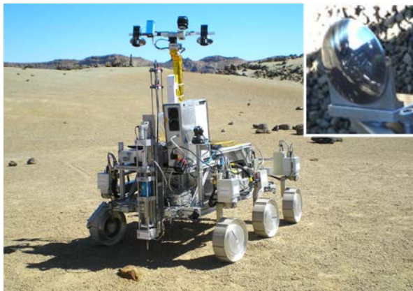
FIGURE 2. A University of Glasgow ultrasonic drill tool undergoing field trials on Mt. Teide, where bit rotation is provided independently of the ultrasonic action through a commutated gearmotor on a splined shaft. Note that drilling is observed (inset) from the twin cameras on the mast via an inspection mirror near the front right wheel.
