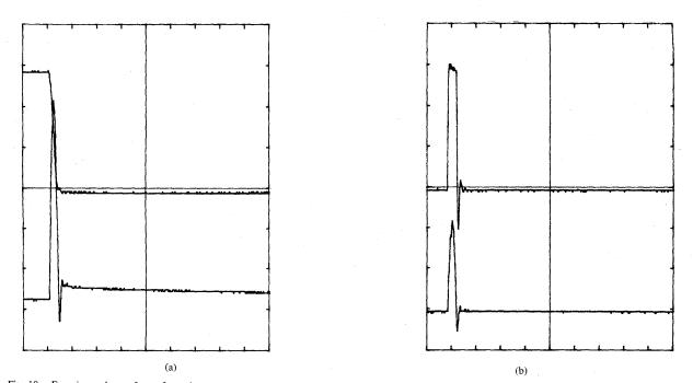
Fig. 10. Experimental waveforms for resistor reset, time base 5  $\mu$ s/division. (a) Upper trace, capacitor voltage (50 V/division); lower trace, primary current (2.5 A/division). (b) Upper trace, secondary voltage (50 V/division); lower trace, secondary current (2.5 A/division).
