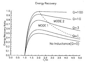
Fig. 4. Curves of the energy recovery ratio  $E_1/E_o$  for varying Q factor and turns ratio. The dashed line shows the boundary between mode 1 and mode 2 recovery.
