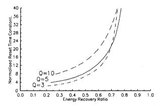
Fig. 6. Normalized reset time constant ( $\omega_0 L_{mag}/2\pi R_s$ ) against energy recovery ratio (m=1/2).
