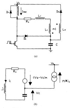
Fig. 5. The modified catch winding energy recovery circuit with resistor reset: (a) circuit and (b) equivalent circuit.
