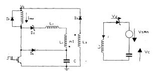
Fig. 7. The catch winding energy recovery circuit with Zener diode  $(D_z)$  reset: (a) circuit and (b) equivalent circuit.
