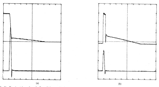
Fig. 11. Experimental waveforms for Zener diode reset, time base 5  $\mu$ s/division. (a) Upper trace, capacitor voltage (50 V/division); lower trace, primary current (2.5 A/division). (b) Upper trace, secondary voltage (50 V/division); lower trace, secondary current (2.5 A/division).
