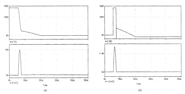
Fig. 9. Pspice simulations for Zener diode reset, m = 0.5. (a) Capacitor voltage v(13) and primary current i(ls1). (b) Secondary voltage v(30) and secondary current i(ls2).
