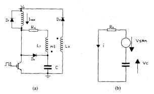
Fig. 2. The catch winding energy recovery circuit with resistor rest: (a) circuit and (b) equivalent circuit.
