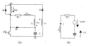
Fig. 3. The improved catch winding energy recovery circuit with resistor reset: (a) circuit and (b) equivalent circuit.
