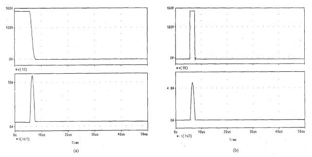
Fig. 8. Pspice simulations for resistor reset, m = 0.5. (a) Capacitor voltage v(13) and primary current i(ls1). (b) Secondary voltage v(30) and secondary current i(ls2).
