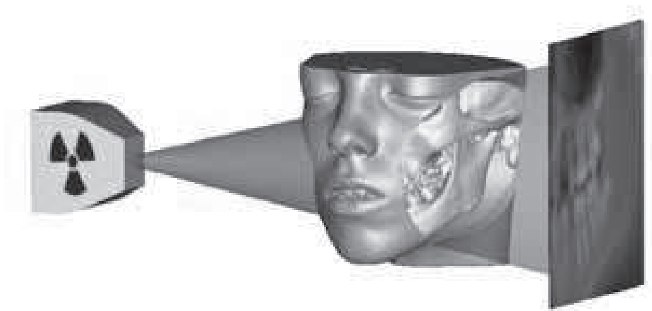
Figure 5 CBCT working process
