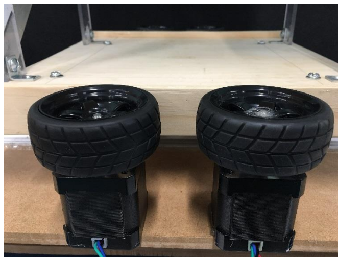
Figure 5-3-2 Stepper Motors and The Base of Structure
