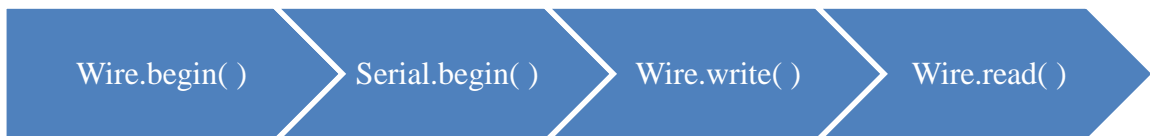
Figure 3-3-1 The Flow Chart of Accelerometer ADXL345
