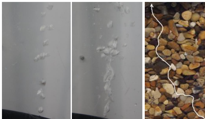
Figure 4.9 Bubble pathways in non-media system (0.8 mm), 15 L/min (left) and 60 L/min (middle) and media system (right)
