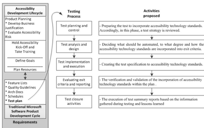
Figure 3. Test process proposed
