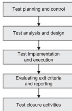
Figure 1. Fundamental Test Process
