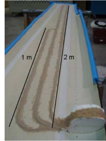
Fig. 4. Picture of the bottom surface of the aircraft flap with the POF fixed to it. The POF, in a loop-shaped configuration, has been installed with two different semilengths of 2 m and 1 m.
