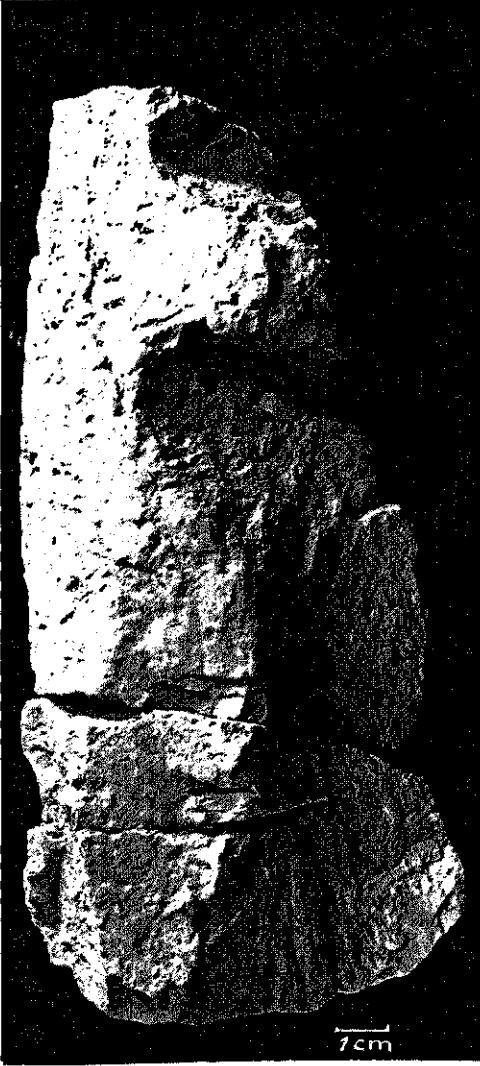
Fig. 52. Smooth single prism from a Playa Marl Soil (100 cm deep in Profile E 1.1). Compare with pedality of the nearby E 1.3 in Figure 64.
