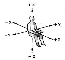
FIG. 17. System of coordinates for mechanical vibrations (I.S.O.; 1967). X-axis: back-chest Y-axis: shoulder-shoulder Z-axis: foot-head
