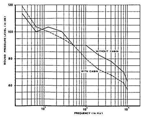
FIG. 16. Sound pressure level of combines.
