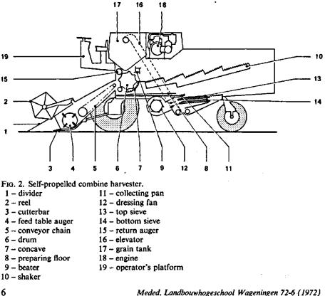
be installed on the platform a pick-up attachment; besides the cutting unit can be exchanged by a unit for picking maize. An auger (4) transports the crop to a conveyor chain (5); this will transport the crop to a threshing mechanism.
