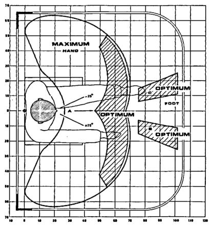
A.1. Optimum work-space lay-out for the self-propelled combine harvester (horizontal plane); 18 cm above seat-reference point (SRP).
