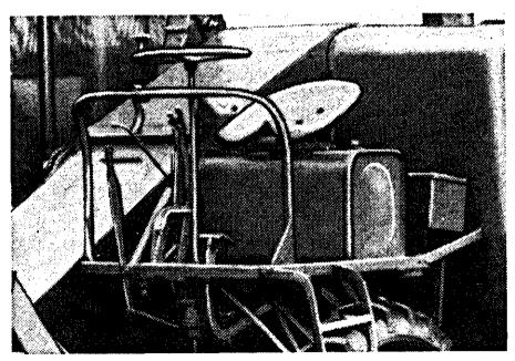
FIG. 8. Work-space lay-out of an old type of combine.
