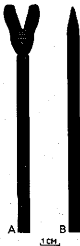
FIG. 33. Longitudinal view of a glass micro-mortar (A) with glass pestle (B).
