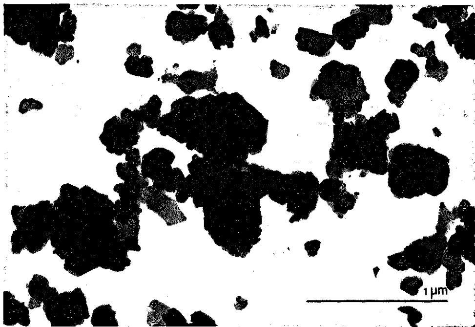
Fig. 16. Electron micrograph of the clay fraction of sample 48 (TFDL).
