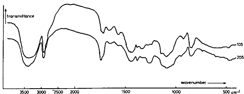
FIG. 3.2-2. IR absorption spectra of Poval 105 and 205.
