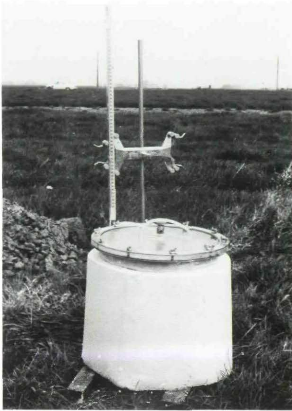
Fig. 24. Measurement of K_{sat} on a large undisturbed soil core which was carved out in situ , set in gypsum and removed from the profile.
