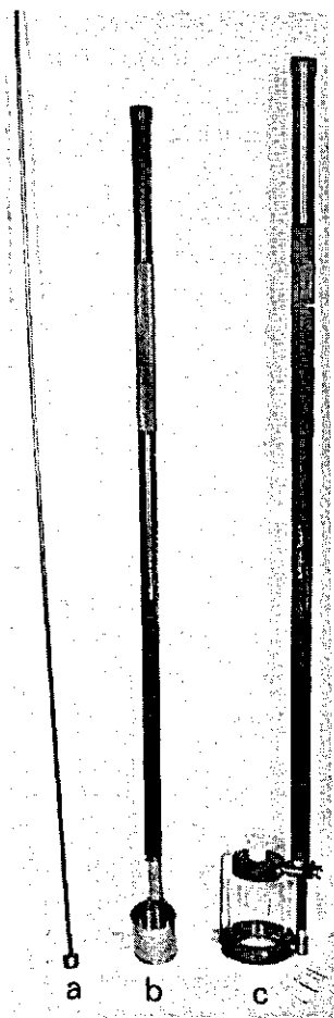
Figure 2. Water sampling devices used in the present study. a. Stainless steel tube used for sampling of drainage ditches and groundwater. b. Stainless steel dip sampler used for sampling of drainage ditches. c. Glass dip sampler used for sampling of large watercourses.
