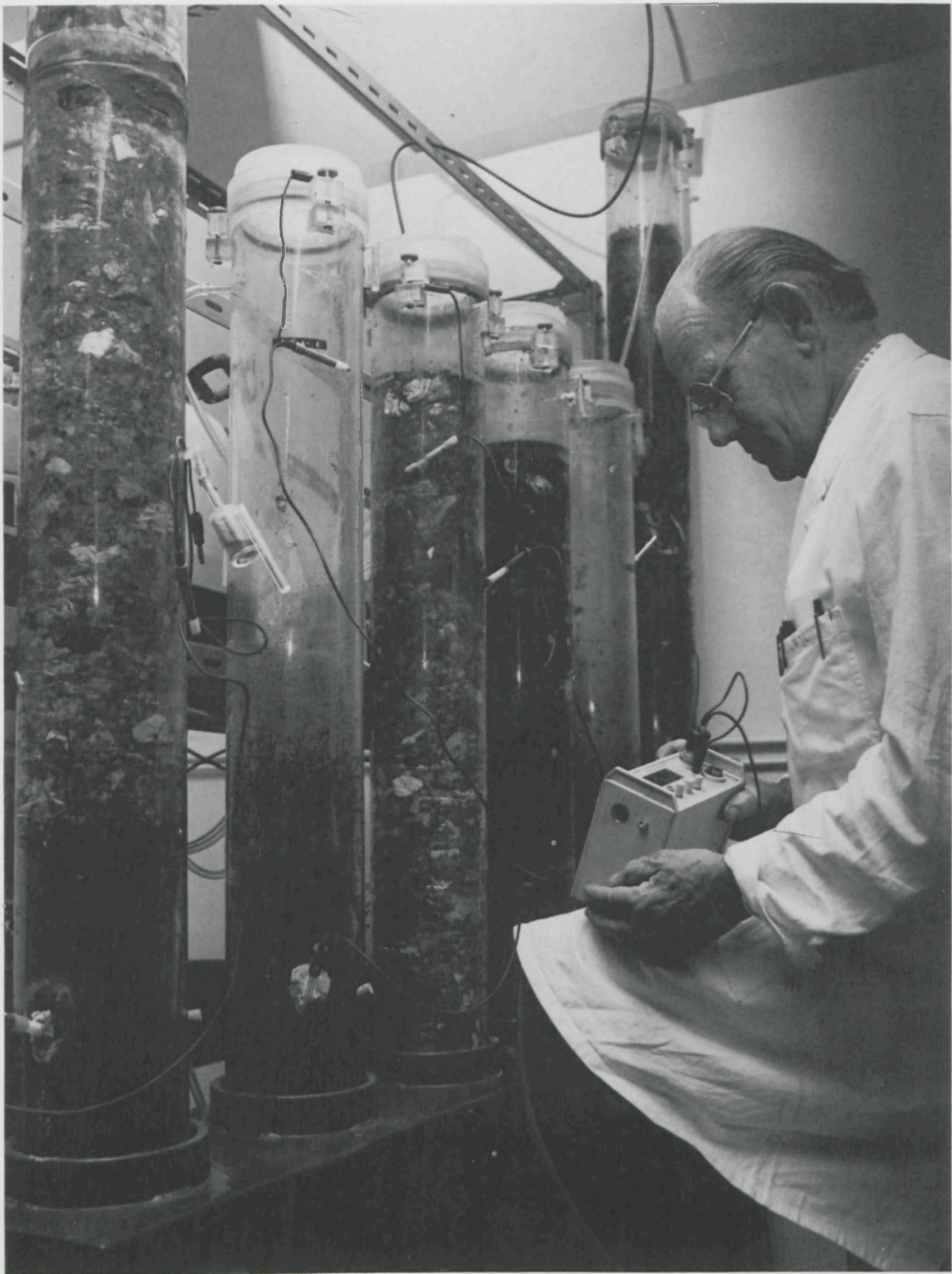
To study transport of materials in the soil they are radio-labelled, so that they can be followed on their way through a soil column.
