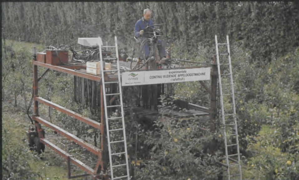
The prototype of a straddle harvester moves over the trees during the harvesting of apples and pears.
