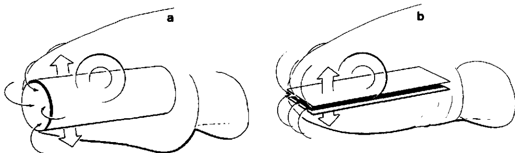
Fig. 1. The mouth cavity of a fish while sucking prey can be approximated by an expanding cylinder (a) or by two plates, initially lying close together and moving away from each other (b).
