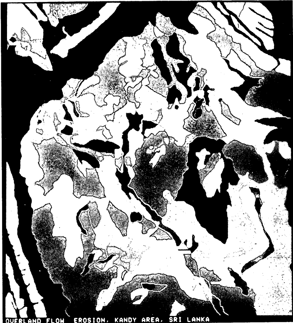
Map 1 Map Showing erosion classes in kg/ha resulting from GIS operation based on Morgan's model. Black and white reproduction of a colour map; dark units low erosion, light toned units higher erosion. Kandy area, Sri Lanka.
