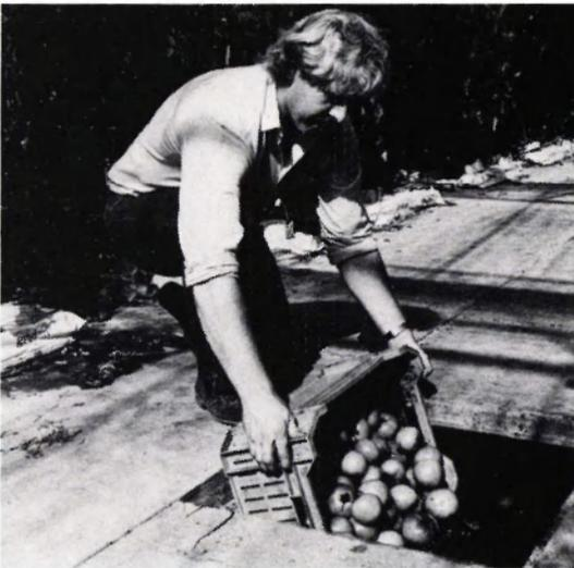
*Water flume system for internal transport*
