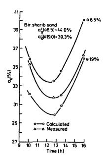
Fig. 4. Surface reflectance measurements
