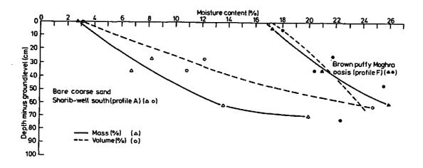
Fig. 9. Moisture versus depth profile
