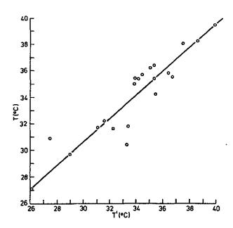
Fig. 2. Calibration data of thermal infrared radiometer;  $\mathbf{T_0}'$ , radiation temperature by means of thermal infrared radiometer;  $\mathbf{T_0}$ , actual temperature of reference black body
