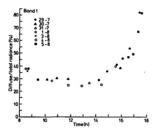
Fig. 6. Ratio of diffuse to total irradiance
