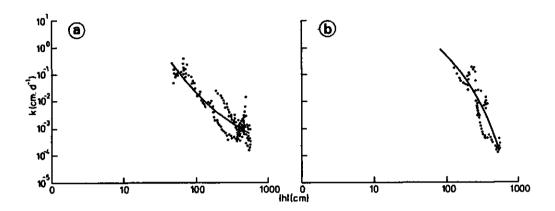
Fig. 10. Unsaturated hydraulic conductivities
