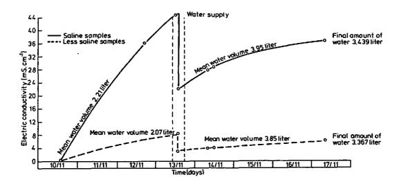
Fig. 11. Salt leaching during saturation process; laboratory experiment
